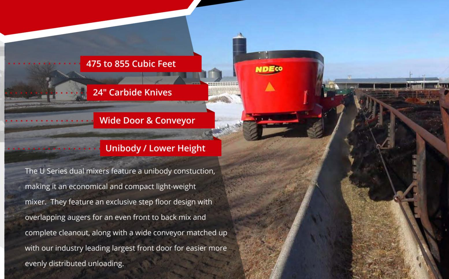
The U Series dual mixers feature a unibody construction, making it an economical and compact light-weight mixer. They feature an exclusive step floor design with overlapping augers for an even front to back mix and complete cleanout, along with a wide conveyor matched up with our industry leading largest front door for easier more evenly distributed unloading.
